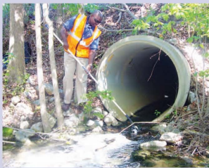
City employee, Dennis McBride, takes a storm water sample from an area drain.
